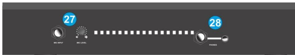
27. **MIC INPUT/LEVEL.** Connect a 1/4" microphone to this input. This input's audio signal is routed directly to the Master Output. Adjust the level/Volume of the Microphone Input, using the knob next to the socket. Hardware Operation, not visible on the VirtualDJ GUI.
