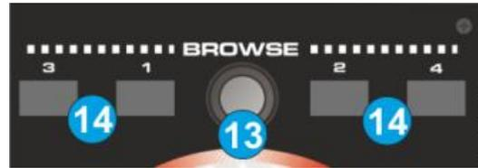
**14. LOAD.** Load the selected track from Browser to the corresponding deck. Hold the same button for more than 1 sec to unload the same deck.
